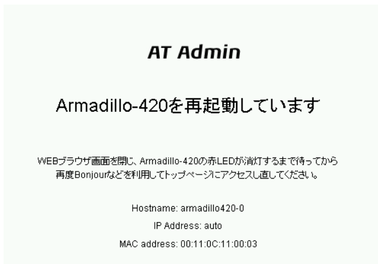
図 4.24 AT Admin: System - Reboot
