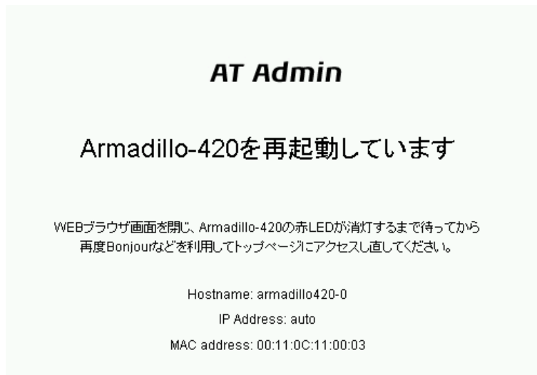
図 4.24 AT Admin: System - Reboot
