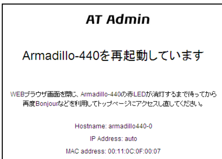
図 6.23 AT Admin: System - Reboot
