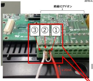
In this connection example, the channel to be measured is "ch0".
